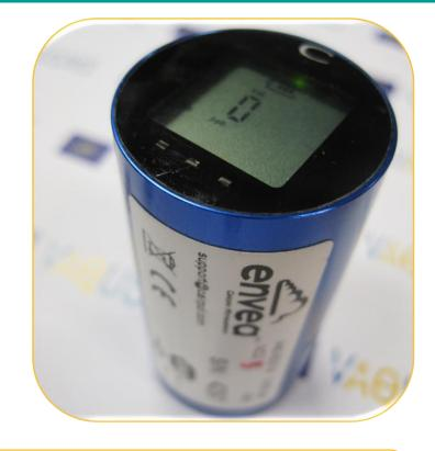
The CairClip  $NO_2$  is a lightweight, portable sensor for measuring nitrogen dioxide in ppb or  $\mu g/m^3$  in applications such as personal exposure and indoor and outdoor air quality monitoring. It uses a micro fan to actively sample air. The CairClip can run on battery power for approximately 24 hours, but it can also operate continuously for much longer periods when plugged into a power source.
